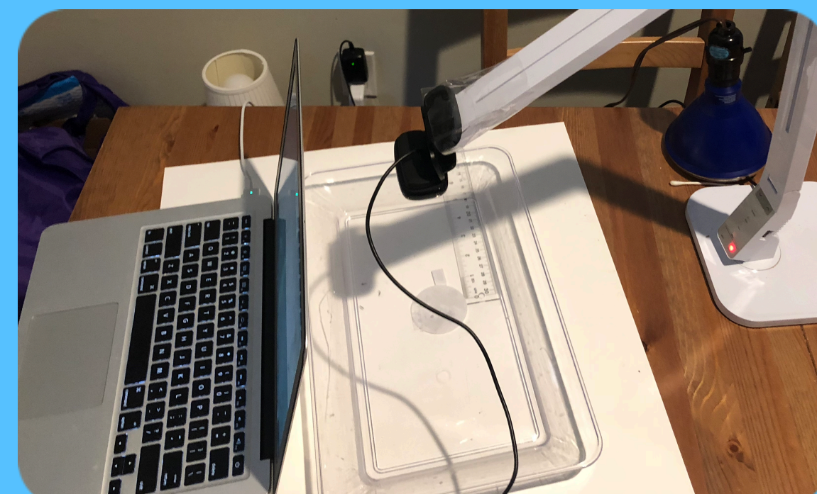
Figure 5b: Filming setup: Logitech C615 Webcam connected to an Apple laptop.
